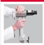
Hydraulic installation tool, compact swage forward design. Installs 14 & 16 mm Huck-Spin Lockbolts.
