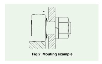
②The IIM□ mark on the flange head of stud indicates the position of oil hole on the raceway. Avoid locating the oil hole within the loading zone. It may lead to short bearing life. (Refer to Fig.3.) The hole located in the middle part of the stud perpendicular to the stud center axis is used for greasing or locking the stud rotation.
