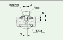
The recommended tolerance of mounting hole for the stud of Heavy Duty Type Cam Follower is H7. Cam Followers are supported in a cantilever position. So, especially when heavy shock loads are applied, the mounting hole diameter should be prepared without play between the stud and the hole.
