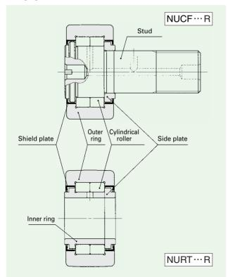
Fig.1 Structure of Heavy Duty Type Cam Follower and Roller Follower
