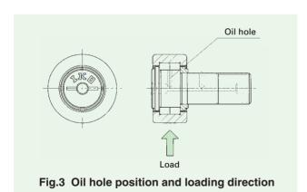
When tightening the nut, the tightening torque should not exceed the maximum tightening torque shown in the dimension tables. If the tightening torque is too large, it is possible that the threaded portion of stud will be broken. When there are possibilities of loosening, a special nut such as a lock nut, a spring washer or a self-locking nut should be used.
